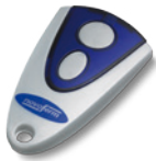
Handsender Micro-Novotron 512 2-Kanal, 433 MHz, KeeLoq-Wechselcode
